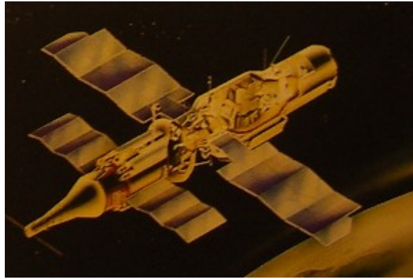
Soviet Salyut (Almaz) Military Manned Space Station: Equipped with a 23mm cannon and designed to withstand combat damage in the vacuum of space. Source: NPO Mashinostroyeniya via RD Fisher
